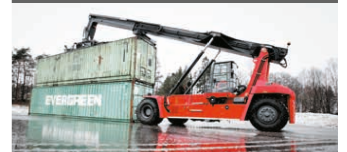
Precise lifting of long container end-on - 40 ft
